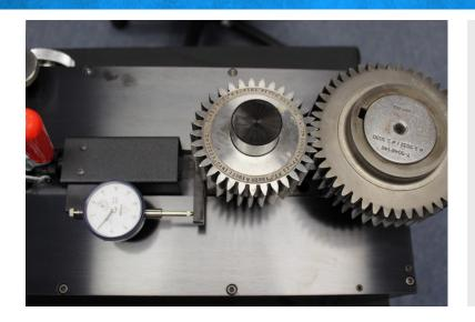
**INSPECTS: Pitch diameter runout**
