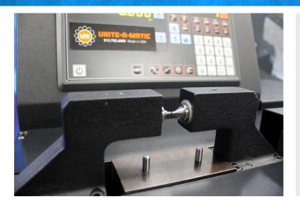
INSPECTS: Pitch diameter (DOB), tip diameter (major), root diameter (minor)
